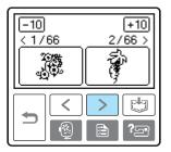
• When -10/+10 is pressed, the display of patterns moves backward/forward 10 patterns.
